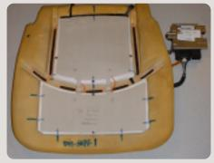
flow within the sensor mat. The ECU algorithm uses this change in current flow to determine the classification of the occupant.
