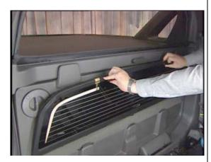
Using the grab handles, pull the rear glass panel out of the storage pocket.
