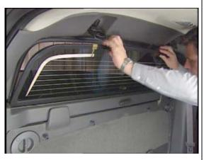
Then, with the rear glass tilted at an angle, place the bottom of the glass panel into the lower channel of the window frame.
