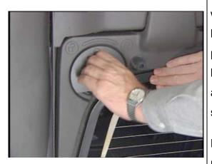
Holding the glass flat against the storage pocket with the grab handles facing you.....Turn both glass lock knobs to the locked position. You may need to push the corner of the glass gently to enable the lock mechanism to engage. Once both lock knobs are in the locked position your rear glass panel is securely stored.
