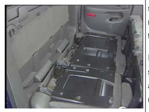
To lower the Midgate panel, first fold down the rear seats. As with removing the rear glass panel, you may have to move the front seat slightly to allow the rear seats to fold completely.
