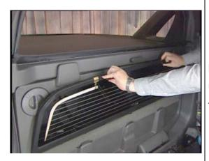
...Then slide the glass panel into the storage pocket located on the back of the Midgate panel using the lower edge of the glass to guide it behind the three glass retaining tabs.
