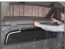
If the rear glass panel is stored in its pocket, stand outside the vehicle and place one hand against the crossbar so the Midgate doesn't fall.
