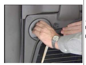
...Then, while holding the glass in place with one hand, turn the glass lock knobs to the unlock position.
