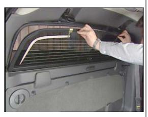
Next, using the two grab handles at the top of the glass... ... Tilt the top of the glass toward you and then lift it out from the lower window frame channel...
