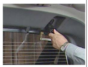
After you have folded down the rear seats, squeeze and pull down the two latch levers located near the upper corners of the rear glass panel.
