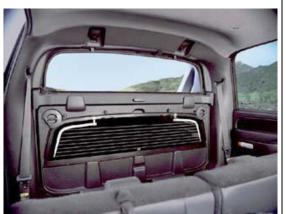
Remember, the Midgate panel on your Chevy Avalanche can be lowered with the rear glass panel in its normal position <u>or</u> with the rear glass panel removed and stowed in the storage pocket.
