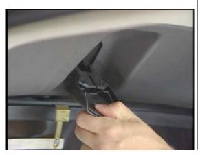
To reinstall the rear glass panel, just squeeze and pull down the latch levers...
