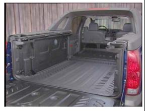
You can open the Midgate with the rear glass in place to create a cargo area that will hold a 4x8 sheet of dry wall or plywood in a weather-resistant area.
