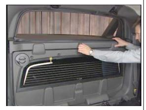
To put the Midgate back into the up position, simply lift it up and firmly push it back into its upright position.
