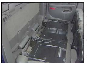
To remove the rear glass panel, first fold down the rear seats completely. It may also be necessary to slide the front seats forward to ensure that you can fold the rear seats down completely.
