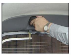
Next, push the rear glass panel against the window frame while applying firm downward pressure. Use the grab handles at the top of the glass to assist you.
