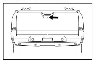
The image is provided by the camera located under the liftgate handle.
