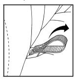
Pull the seat loop located where the seatback and seat cushion meet. The seat cushion will release and allow you to tilt it toward the front of the yehicle.
