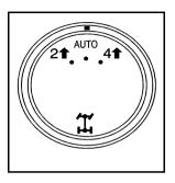
The transfer case knob is located to the left of the instrument panel cluster.
