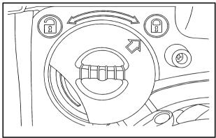
Turn both glass lock knobs (D), located at both top corners of the storage pocket, to the locked position. Push in on the corner of the rear glass to allow the lock knob to engage more easily. Once both glass lock knobs are in the locked position, the rear glass is securely stored.
