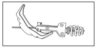
Tilt the tire. Separate the tire/wheel retainer (D) from the guide pin. Pull the pin through the center of the wheel. Tilt the retainer down through the center wheel opening.
