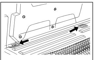
The cargo net has cut outs for the four cargo-area floor drains located under the cargo mat near the sides of the cargo area.
