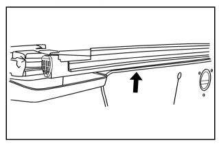
The side rail channels are located on top of both sides of the cargo area. Flush them out with clean water if debris collects inside of them.
