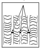
One way to tell when it is time for new tires is to check the treadwear indicators, which appear when your tires have only 1/16 inch (1.6 mm) or less of tread remaining. Some commercial truck tires may not have treadwear indicators
