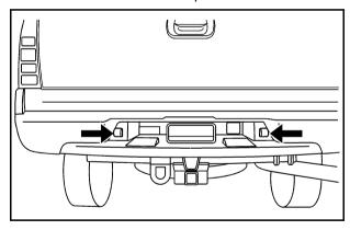
Turn the bulb socket counterclockwise and pull the bulb socket out of the connector.
