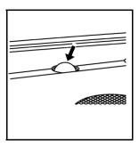
The solar sensor, located in the defrost grille, middle of the instrument panel, monitors the solar heat. Do not cover the solar sensor or the system will not work properly.
