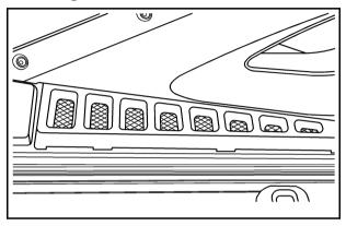
The top drain grates are located near the rear window on both sides of the vehicle. Clean the grates and drains if there is a blockage. To remove each drain grate, do the following:
