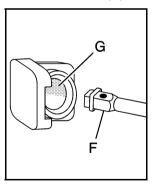
Insert the open end of the extension (F) through the hole in the rear bumper (G) (hoist shaft access hole).
