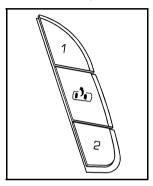
The controls for this feature are located on the driver door, and are used to program and recall memory settings for the driver seat, outside mirrors, and the adjustable throttle and brake pedal feature.
