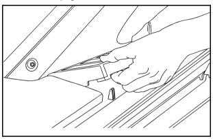
2. Grasp the edges of the grate and pull it out from the vehicle. Flush the drain with clean water.
