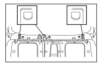
The top tether anchors are located on the back of the rear seat frame above the floor for each rear seating position. Fold down the rear seatback(s) to access the anchors. See *Rear Seat Operation on page 2-13*. Be sure to use an anchor located on the same side of the vehicle as the seating position where the child restraint will be placed.
