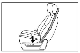
If equipped, this control is located on the outboard side of the seat.
