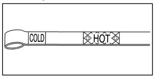
Safe operating level is within the HOT cross hatch band on the dipstick. If the fluid level is not within the HOT band, and the transmission temperature is between 160°F and 200°F (71°C and 93°C), add
