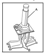
Place the bottom edge of the jack (A) on the wheel blocks (B), separating them so that the jack is balanced securely.
