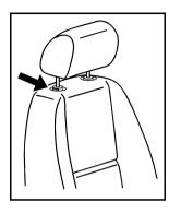
Pull the head restraint up to raise it. To lower the head restraint, press the button, located on the top of the seatback, and push the restraint down.
