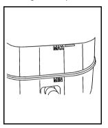
The fluid level should be above MIN. If it is not, have the brake hydraulic system checked to see if there is a leak.
