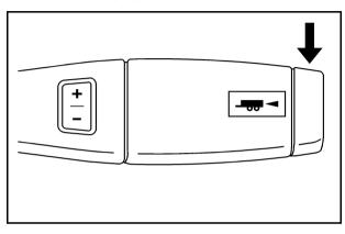
The vehicle has a tow/haul mode. The tow/haul mode adjusts the transmission shift pattern to reduce shift cycling, providing increased performance, vehicle control, and transmission cooling while towing or hauling heavy loads.
