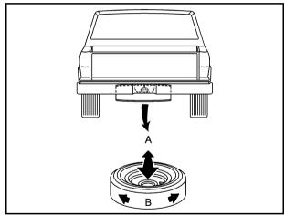
Make sure the tire is stored securely. Push, pull (A), and then try to turn (B) the tire. If the tire moves, use the wheel wrench to tighten the cable.
