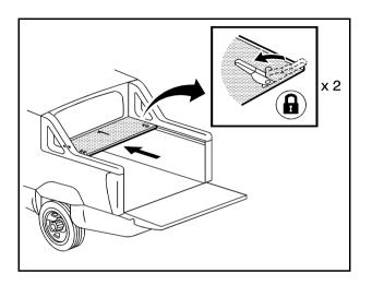
The driver side cargo cover panel latch must lock in place before the passenger side latch can be locked. If this procedure is not followed exactly, the
