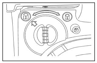
Hold the rear glass in place with one hand and turn the glass lock knobs, located at both top corners of the glass storage pocket, to the unlocked position. 3. Pull the rear glass out from the storage pocket using the grab handles.
