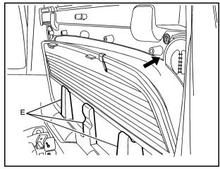
Load the rear glass into the storage pocket in the Midgate<sup>®</sup>, guiding the lower edge of the rear glass behind the three rear glass retaining tabs (E).
