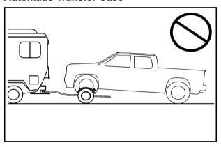
Notice: If a two-wheel drive vehicle or a four-wheel drive vehicle with a single speed automatic transfer case is towed with the rear wheels on the ground, the transmission could be damaged. The repairs would not be covered by the vehicle warranty. Never tow the vehicle with the rear wheels on the ground.
