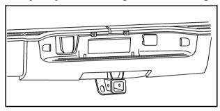
The vehicle has a seven-pin universal heavy-duty trailer connector attached to the rear bumper beam next to the integrated trailer hitch.
