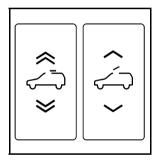
There are two switches in the overhead console that operate the sunroof. Manual-Open/Manual-Close: To open the sunroof press and hold the rear of the driver's side switch until the sunroof reaches the desired position. To close the sunroof, press and hold the front of the driver's side switch until the sunroof reaches the desired position. The sunshade will open automatically with the sunroof, but can also be opened manually.
