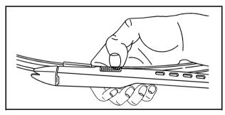
Squeeze the grooved areas on each side of the blade, and rotate the blade assembly away from the arm connector.
