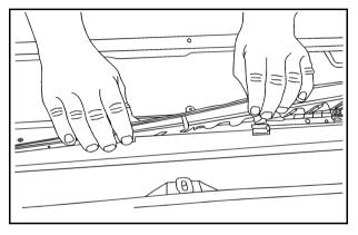
2. Pull up on the rear side of the drain grate, tilt it toward the front of the vehicle, and pull it out.
