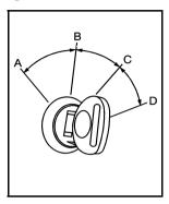
The ignition switch has four different positions.
