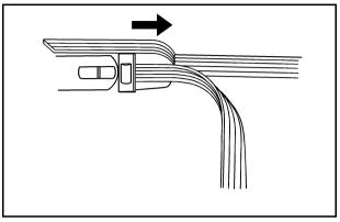
4. Tighten all straps by pulling on the free end of each strap.
