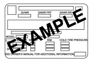
A vehicle specific Certification/Tire label is attached to the rear edge of the driver's door. The label shows the size of your vehicle's original tires and the inflation pressures needed to obtain
