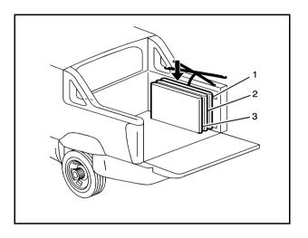
Starting with cargo panel 1, load the cargo panel with the latches facing up toward the side of the cargo box.
