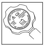
1 You can remove the coolant surge tank pressure cap when the cooling system, including the coolant surge tank pressure cap and upper radiator hose, is no longer hot.
