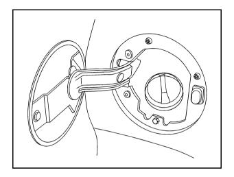
The tethered fuel cap is located behind a hinged fuel door on the driver side of the vehicle. If the vehicle has E85 fuel capability, the fuel cap will be yellow and state that E85 or gasoline can be used. See *Fuel E85* (85% Ethanol) on page 6-8.
