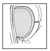
The instrument panel fuse block access door is located on the driver side edge of the instrument panel.
