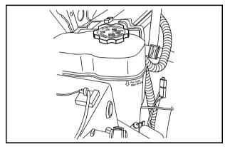
The coolant surge tank is located in the engine compartment on the passenger side of the vehicle. See *Engine Compartment Overview on page 6-14* for more information on location.
