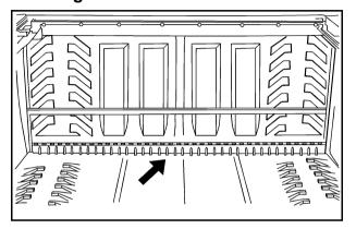
The removable Midgate drain grate is located near the base of the Midgate.
