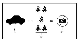
Refer to your vehicle's tire and loading information label for specific information about your vehicle's capacity weight and seating positions. The combined weight of the driver, passengers and cargo should never exceed your vehicle's capacity weight.
