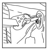
Secure the storage strap system in the cargo storage area by attaching the six clips included on the cargo strap system to the tie down locations on either side of the storage area.
