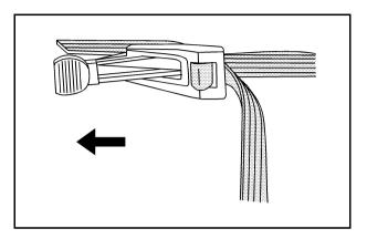
5. Close both cross locks at the center of the strap system to tightly secure.
