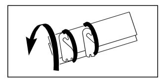
Take the storage strap and wrap it around the package. Finally, attach the hooks to the webbing and place the straps inside the top box storage compartment.
