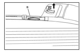
Push the rear glass flat against the window frame and push each latch lever up until it locks. You should hear a click when each latch lever locks correctly.
