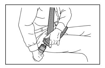
3. Push the latch plate into the buckle until it clicks. If you find that the latch plate will not go fully into the buckle, see if you are using the correct buckle.
